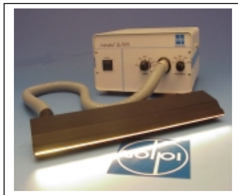
d) Line Converter with Light Source
